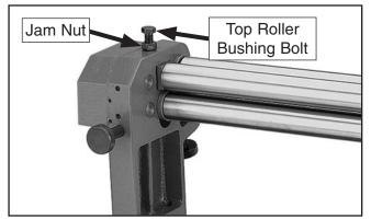
Figure 13. Top roller bushing.
